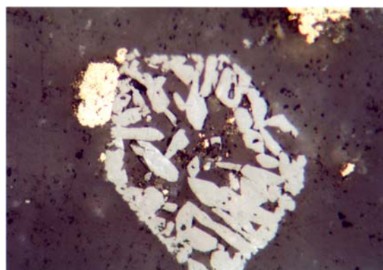
Fig.5. Prismatic and elongated rutile crystals after ilmenite, subhedral pyrite. Au: 10.9 g/t. R377-104m, hydrothermal breccia. Reflected light, 1N.
