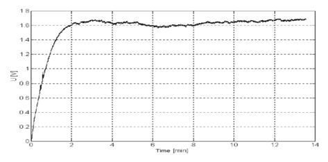
Fig. 3 Transient unit response of the controlled object
