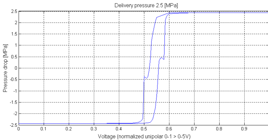
Fig.8. Dependence between pressure drop and voltage.
