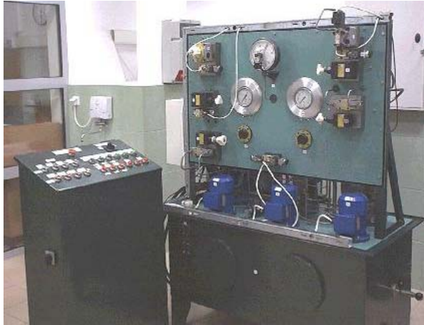
Fig.5. Laboratory stand of the hydrostatic transmission.
