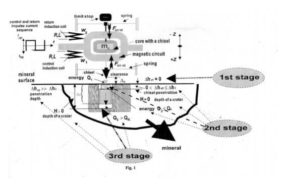
First technological stage. In this case chisel takes out the working clearance  $\Delta_H$  and just touches the surface of the mineral, the penetration into mineral absent  $(\Delta h_d=0)$ .
