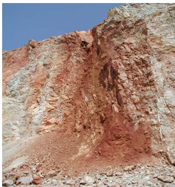
Fig. 46. Subvertical dislocation zone filled by tectonic breccias and bauxite on 10A storey.
