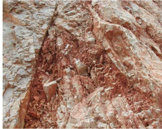
Fig. 38. Tectonic breccias in contact with duplex structure.
