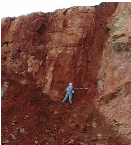
Fig. 45. Suvertical dislocation zone filled by tectonic breccias and bauxite on the 9C storey.
