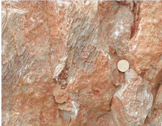
Fig. 37. Lineation of overthrust L=148/54^\circ in the area of duplex structure.
