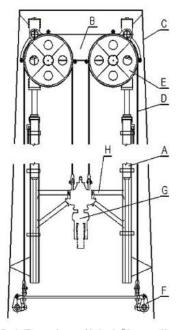
Fig. 1. The main elements of the RamRig<sup>®</sup> hoist assembly, showing the yoke (A), dolly (B), top drive (C), equalizer assembly (D), lifting wires (E) and the ramcylinders (F)
