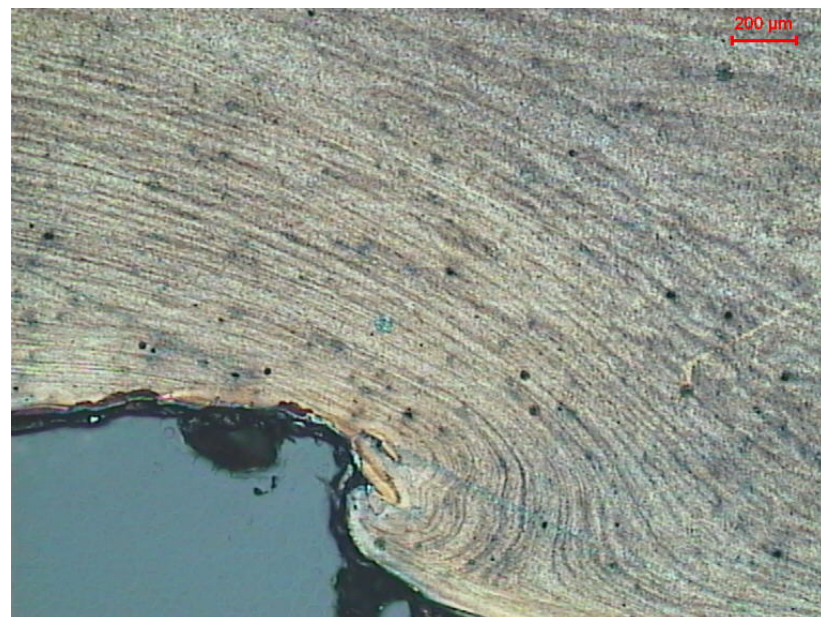
Fig. 10. Strongly deformed surface of the nut. Sample no. 5.
