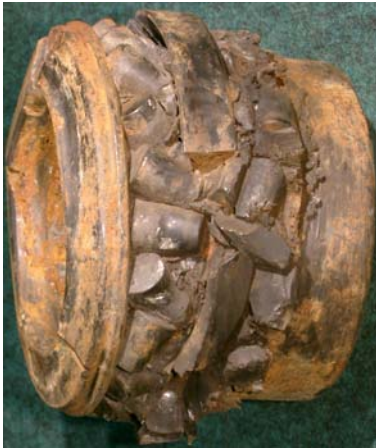
Fig. 7. Elements of bearings fixed at the end of the shaft.
