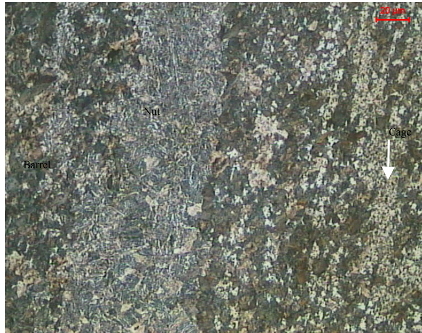
Fig. 9. Structure of the zone of welding of bearing cage, nut and barrel. Visibly mixed materials. Sample no. 2.
