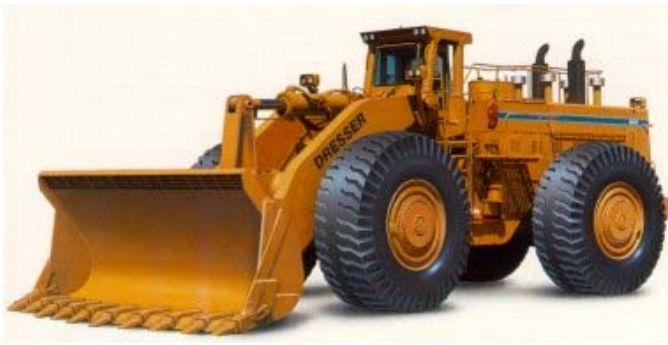
Fig. 4. Loaders on wheel and caterpillar chassis used in open-pit mining.
