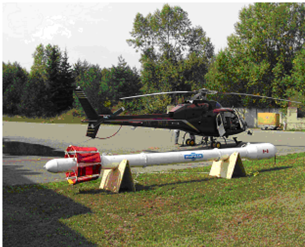
Fig. 3. Electromagnetic system in the gondola prepared for a flight..
