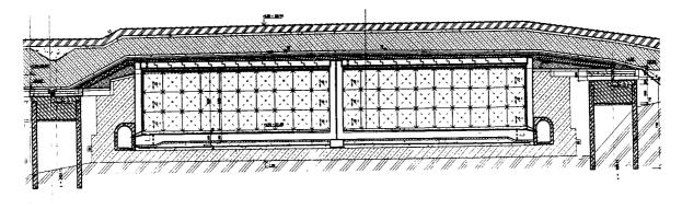
Fig. 2. Schematic cross section of the twins of underground chambers in a definitive container's storage position.
