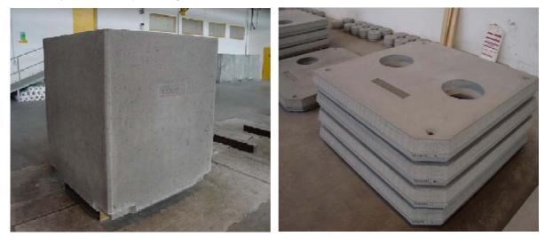
Fig. 6. Precast container body and cover plates made of HPFRC.
