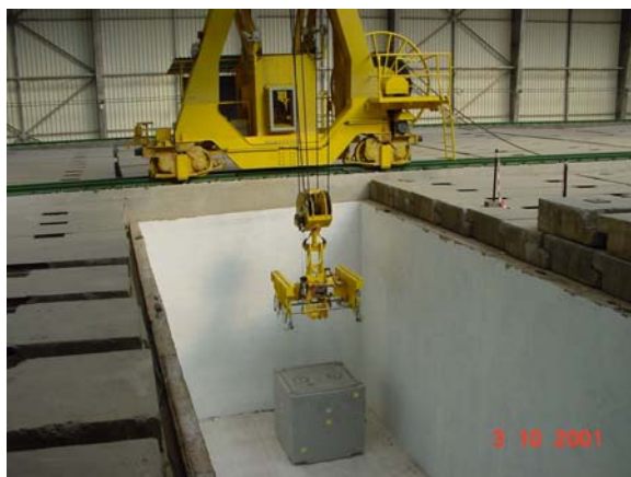
Obr. 3. Zakladanie kontajnera do boxu. Fig. 3. Put of the container in the box.
