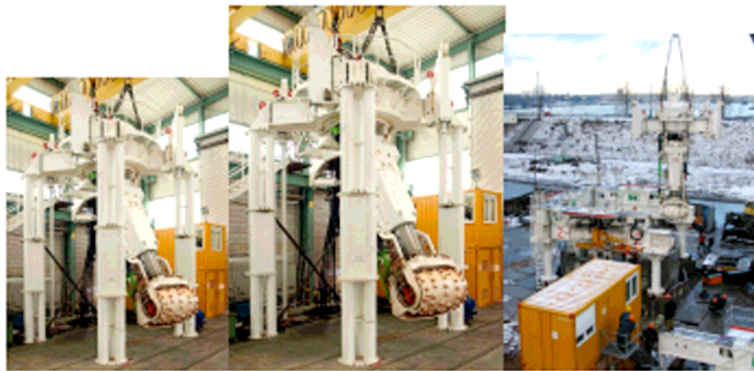
Fig. 8. Shaft sinking equipment in Schwanau - Assembly in St. Petersburg.
