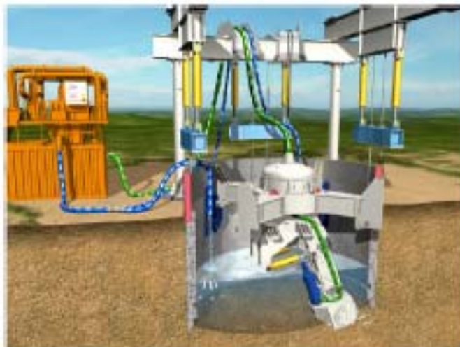
Fig. 1. Structure of the shaft sinking equipment with the shaft sinking and boring unit.
