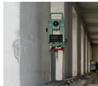
Fig. 2. Leica TCR 305 fastened at rail.
