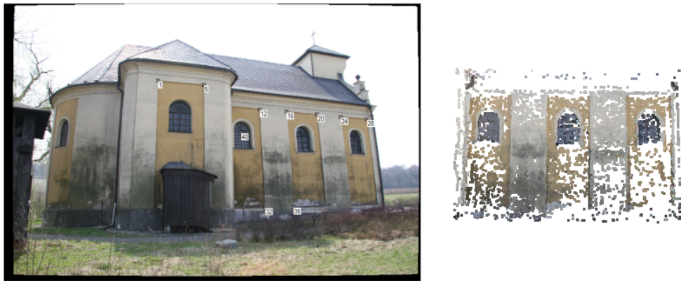
Fig. 8. This image is a screen shot of Photomodeler Idealize Module and Scanner showing a textured 3D point cloud.
