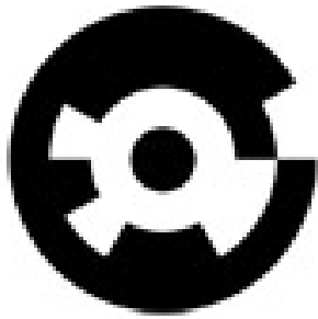
Fig. 7. A Photomodeler Scanner coded target.
