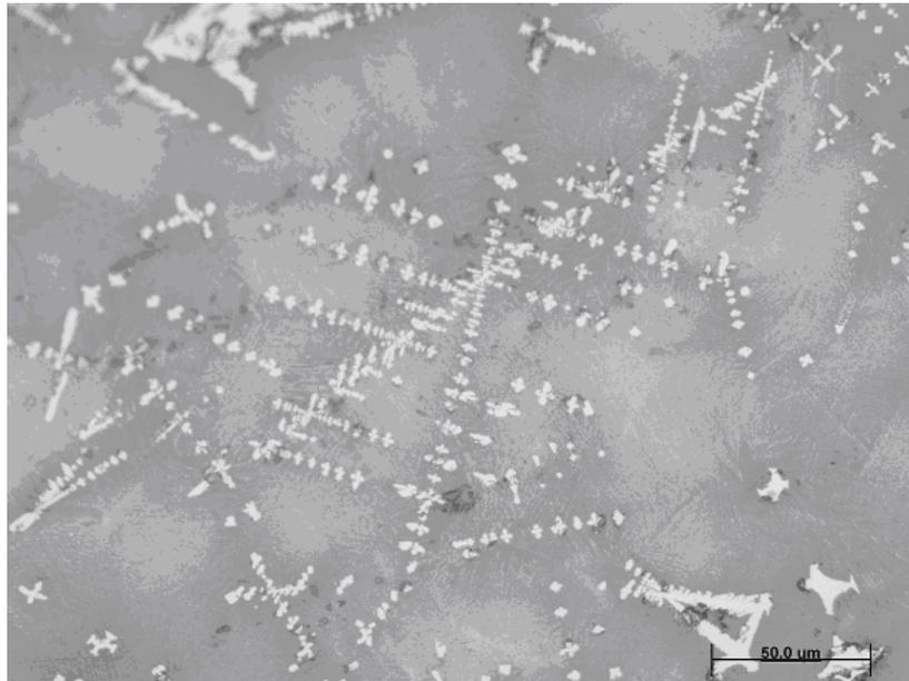
Fig. 1. Dendritic structure - sample 6G.
