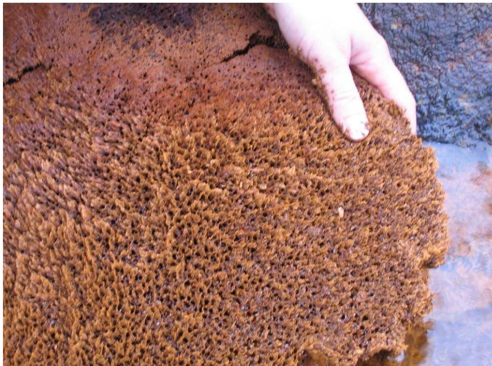
Fig. 3. A sample of ochreous precipitate formed at the AMD discharge from the shaft Pech in the Smolník abandoned mine.
