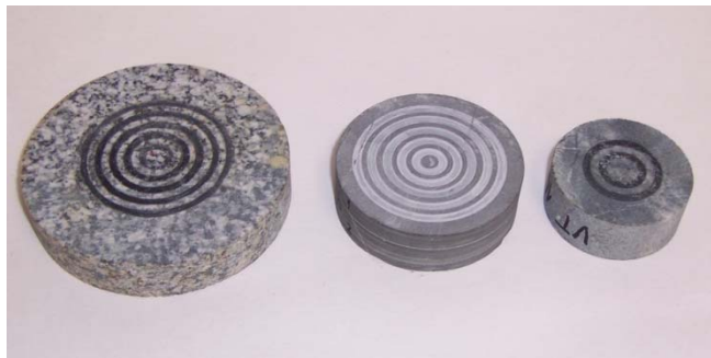
Fig. 8. Rock samples after testing, from left: granodiorite and limestone with five concentric tracks and a smaller sample of gneiss with two tracks.
