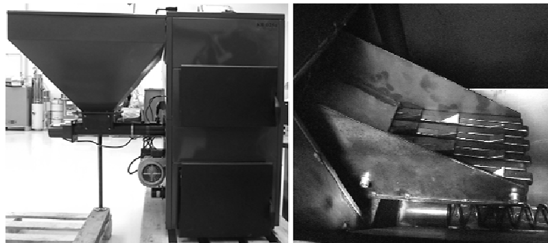
Fig. 1. Left: Boiler “1” for combustion of various pellets, Right: Burner of boiler “1”.
