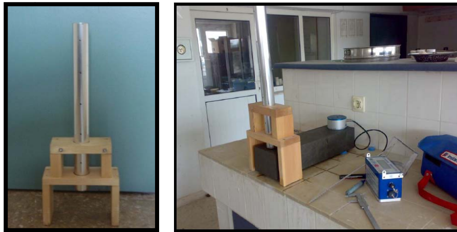
Fig. 3. Vibration wave was generated with especially designed simple but effective instruments shown here. The photo on the right hand site shows the test sample and apparatus just before the test.
