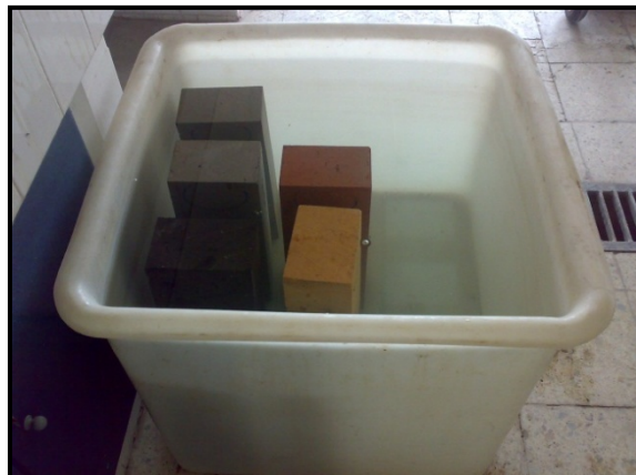
Fig. 2. Rock samples prepared in given dimensions had been kept in water for 48 hour to obtain saturated rock sample condition.
