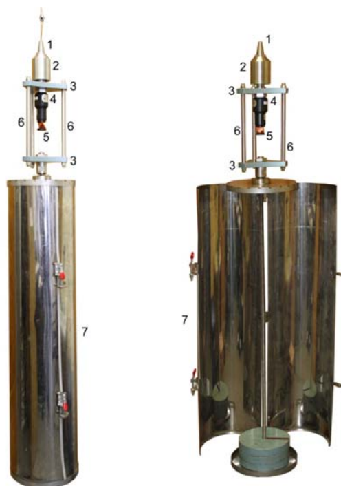
Fig. 1. Suspension for an omnidirectional prism coaxially inserted above the plummet.
