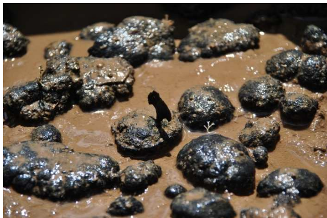
Fig. 2. Polymetric nodules extracted in the Clarion - Clipperton area in the Pacific Ocean (www.5).
