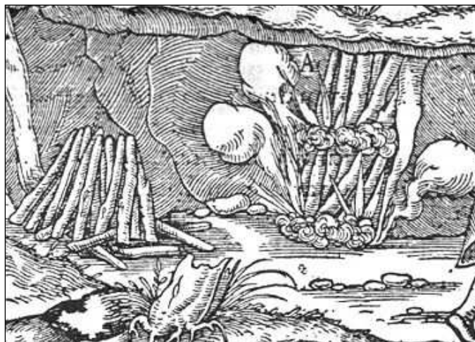
Fig. 11. Firesetting in the 16th century (Agricola 1556).
