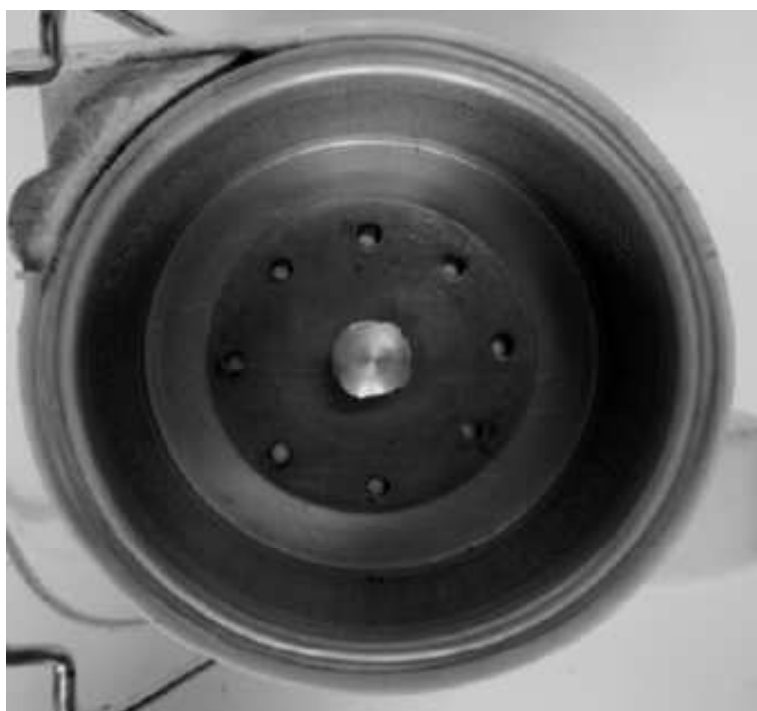
Fig. 5. General view of the perforated drum assembly removed from the experimental stand cover.
