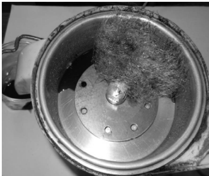
Fig. 6. A typical violation of the perforated drum balancing.
