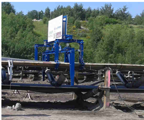
Fig. 4. View of the measurement frame mounted on conveyor Gbf 50 (B2000).
