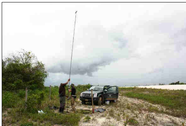
Fig. 2. Exploratory drilling at the Spanish Lookout deposit using a hand-held Eijkelkamp auger set.
