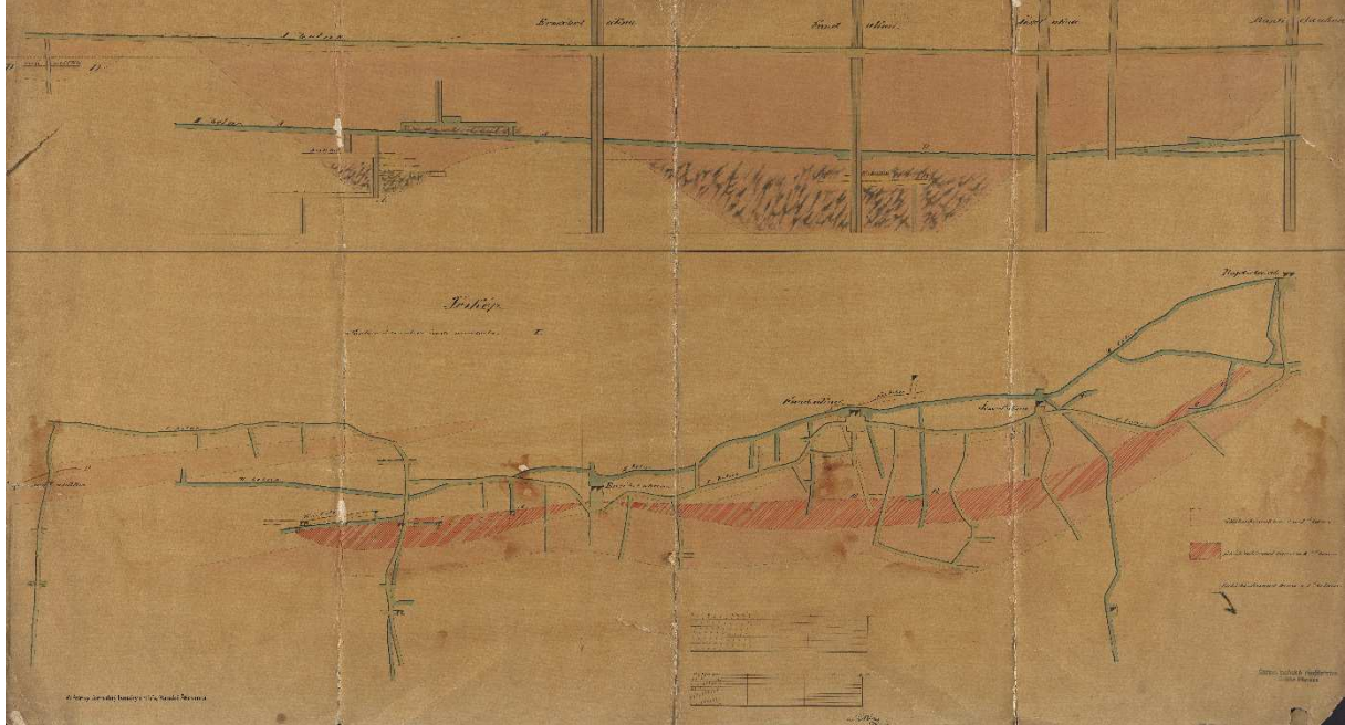
Fig. 7. Mine map from the early 19th century showing the underground for cementation water mining in the mining field in Ostrý vrch hill (Spitzen Berg) (Slovak Mining Archive Banská Štiavnica).
