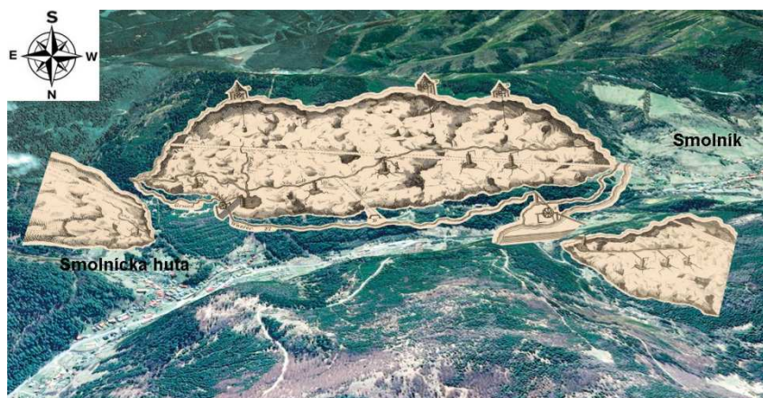
Fig. 4. Projection of the georeferenced Marsigli's map from 1696 into a 3D Google Earth map. The 2D model creates a real and fairly accurate picture of the position of underground passages, underground technological facilities, and surface cementation facilities at the end of the 17th century.
