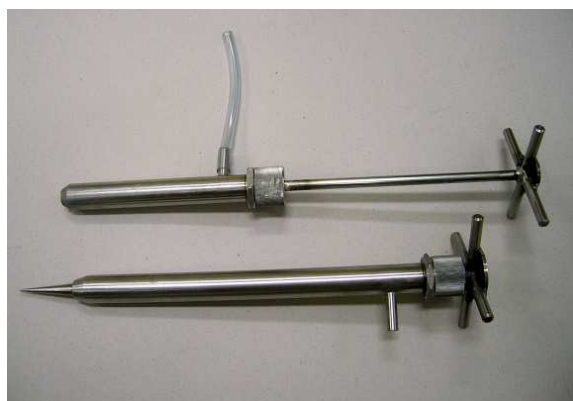
Fig. 2. 16 cm long soil gas probe.
