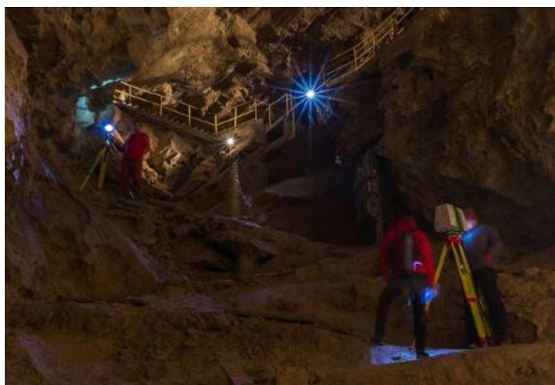
Fig. 2. Leica ScanStation C10 at the survey station during orientation to 6" HDS target.
