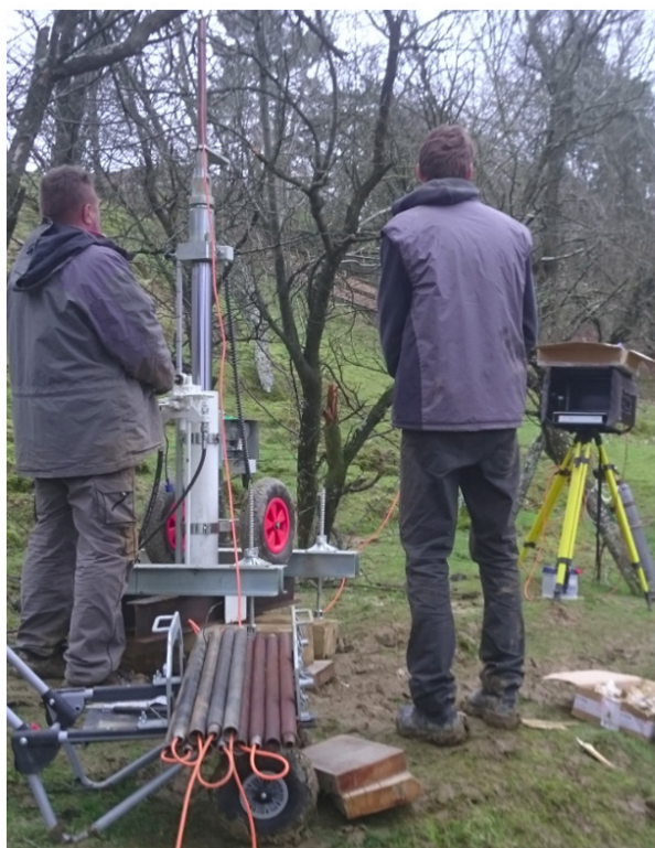
Fig. 6. Portable equipment for static probing, CPTu, on site.
