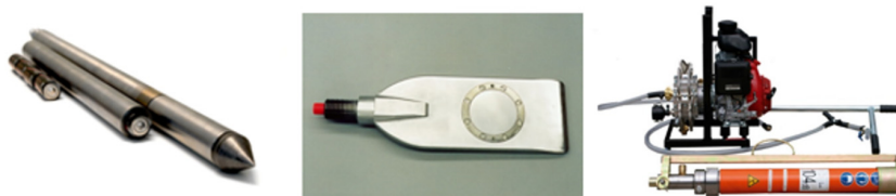
Fig. 9. CPTu penetrometer cone - left, DMT blade - middle, DPL pneumatic ramming device- right.
