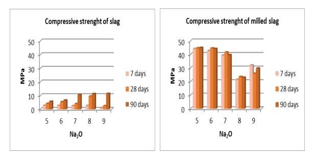
Fig. 4. Compressive strengths of BFS and GGBFS.
