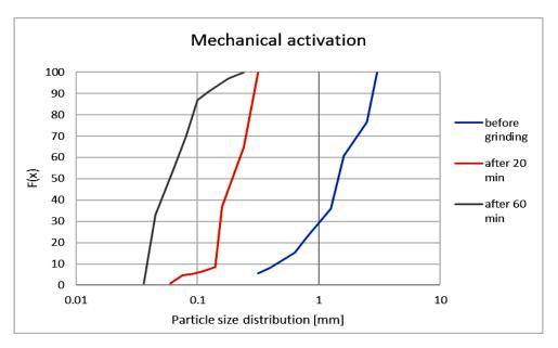
Fig. 1. Particle size distribution before grinding and after 60 minutes of grinding.
