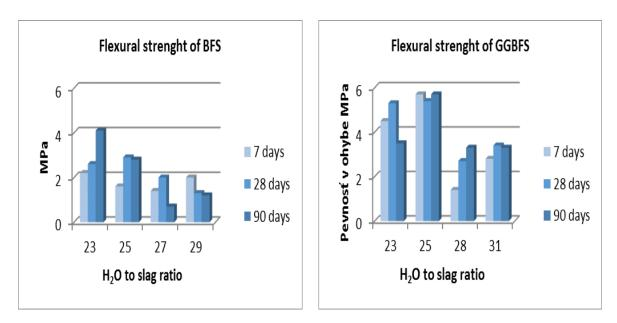
Fig. 7. Flexural strengths of BFS and GGBFS
