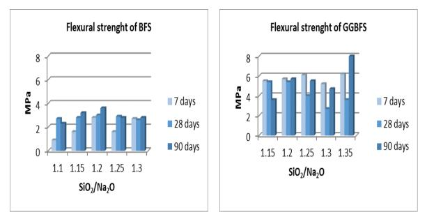
Fig. 5. Flexural strengths of BFS and GGBFS.
