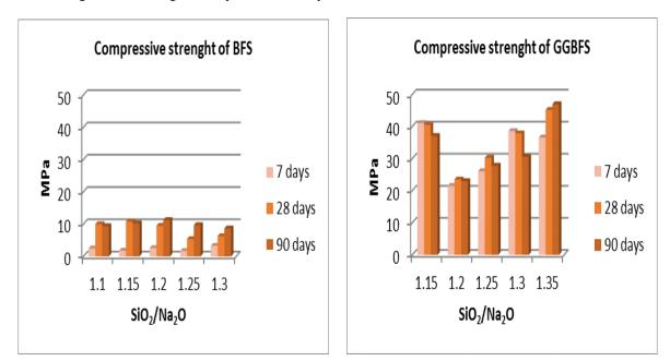
Fig. 6. Compressive strengths of BFS and GGBFS
