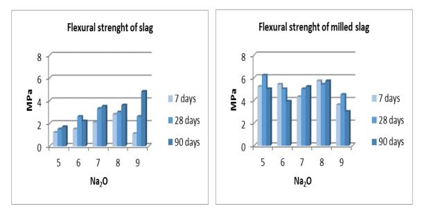
Fig. 3. Flexural strengths of BFS and GGBFS.
