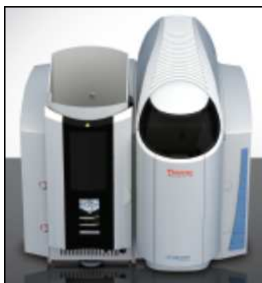
Fig. 3. Thermo Scientific iCE 3300 AA Spectrometer.
