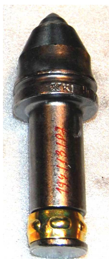
a/ conical pick used in cutting drum of a longwall shearer
