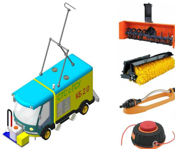
Fig. 1. Hybrid special vehicle with attachable equipment set.
