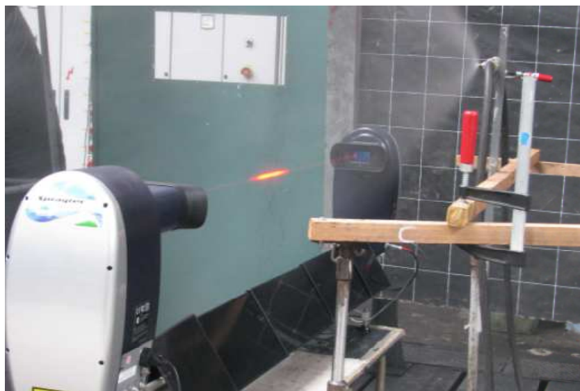
Fig. 4. The test stand during measurements of the distribution of drops diameters in a stream generated by PF250 nozzle (Balaga, 2015)
