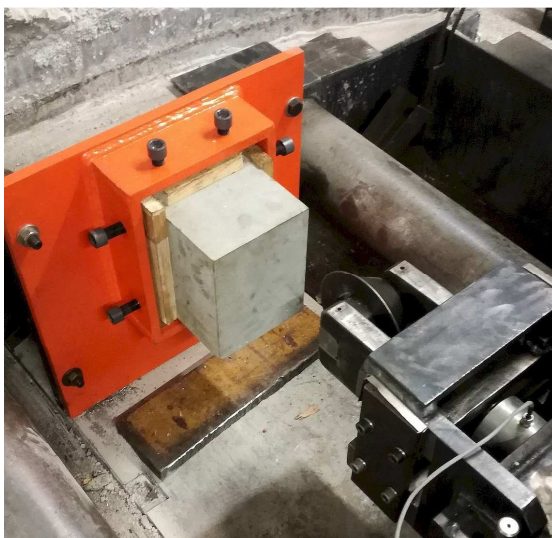
Fig.7. Lab stand for testing mining process of single disc tools
