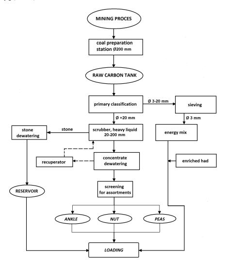
Fig. 2. Technological diagram of coal production
