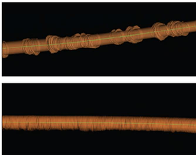
Fig. 1. Comparison of the wellbore quality built according to the calliper data: top - downhole motor with a bent sub, bottom - rotary steerable system.
