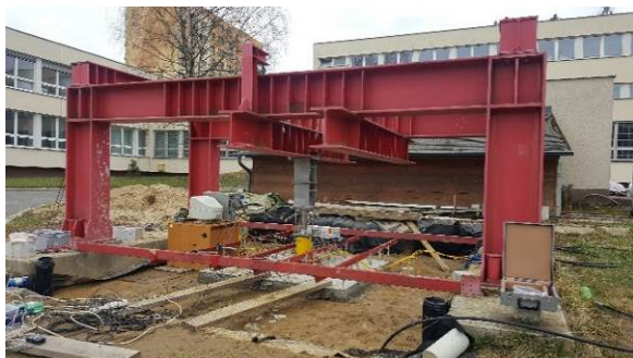
Fig. 2. Stend – steel frame
