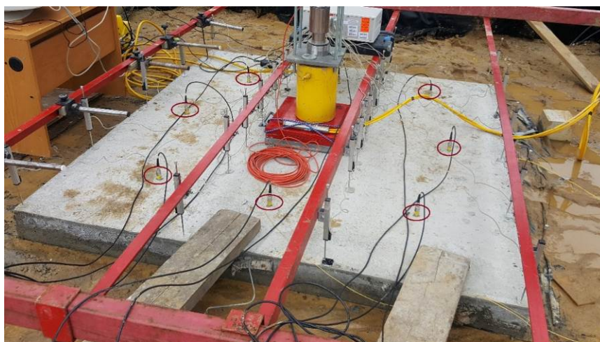
Fig. 9. Concrete slab – during the test: AE sensors
