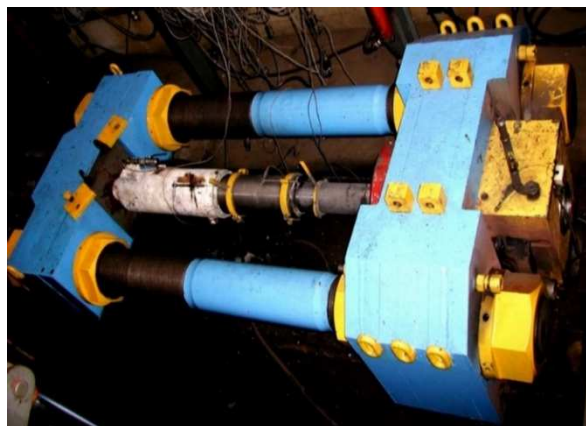
Fig. 3. Facility for testing the legs at dynamic load generated by the explosive method (Madejczyk, 2019)
