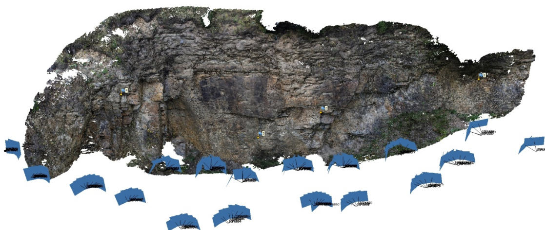
Fig. 6 Ground control points in Bachledova valley and the camera capture positions
