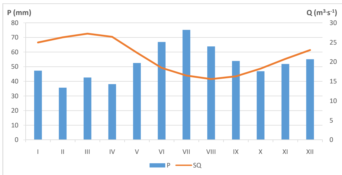
Fig. 5. Average monthly sums of precipitation (P) and average monthly discharges (SQ) of the Drawa River in the Drawiny profile in 1971–2015
