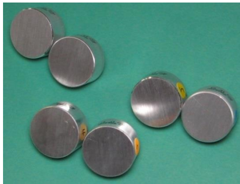
Fig. 4. Selected ultrasonic transducers
