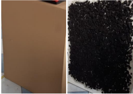
Fig. 7. Flat and uneven coal surface used for testing
