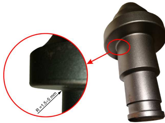
Fig. 4. View of the transition area between the shank and the shoulder of a typical conical pick
