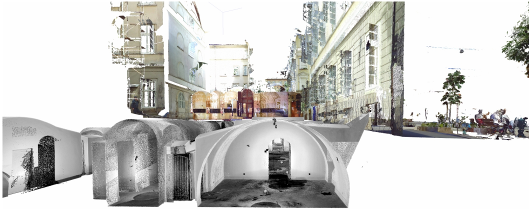
Fig. 7. The point cloud of the Underground Tourist Route and the Main Market Square in Rzeszow coloured with RGB values. Source: own study.
