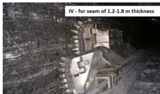
Fig. 2. Plough system applied in the Bogdanka Mine
