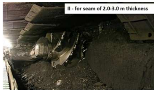
Fig. 1. Longwall system with the use of a shearer at the Bogdanka Mine
