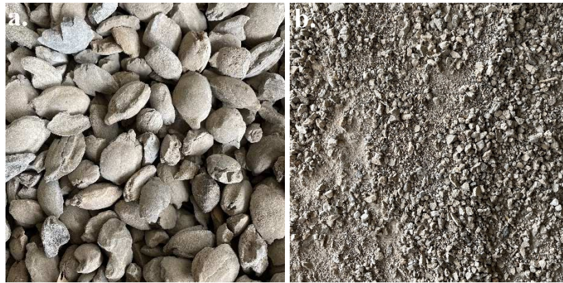
Fig. 1. Appearances of optimized magnesium slags: a. coarse slags, b. fine slags
