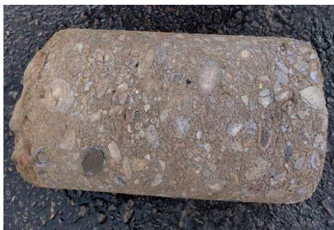
Fig. 10. 7 d core sample from the testing section
