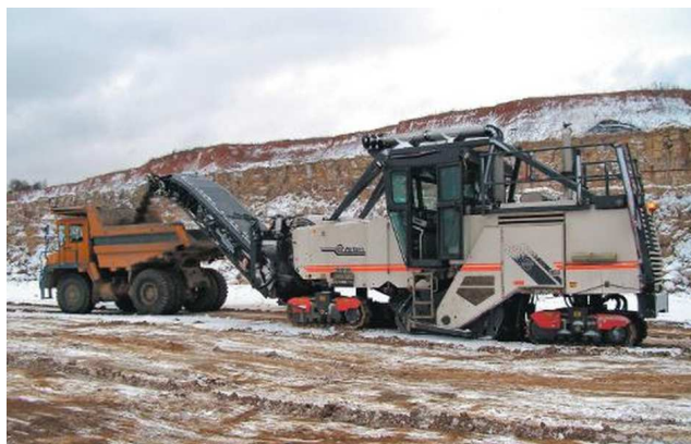
Fig. 1. Wirtgen 2200 SM milling-type excavation and loading machine in Kuzbass
