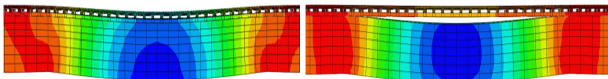
Fig. 7. Track structure deformation caused by differential settlements of subgrade.
