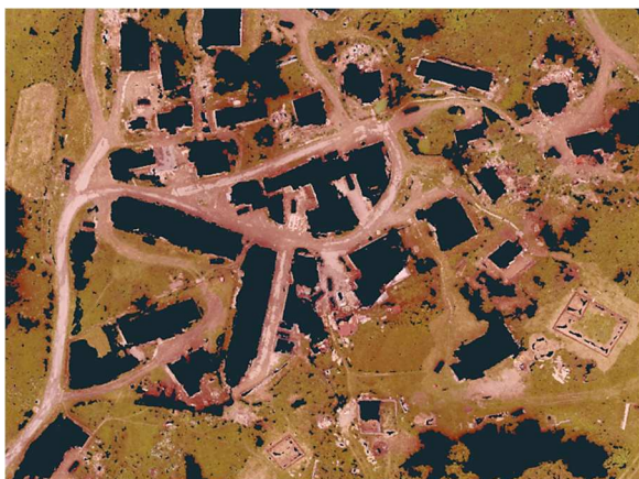
Fig. 12. Classified point-cloud for DTM
