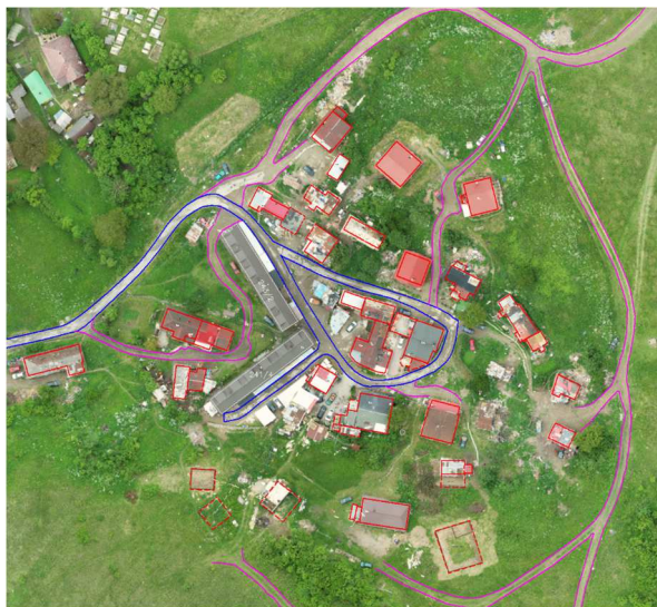
Fig. 10. Orthophoto supplemented by vectorized drawing
