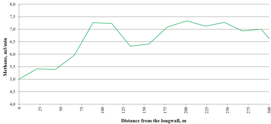
Figure 10. Changes in methane emissions removed through the bleeder road with an increase in the distance from the longwall face to the crosscut
